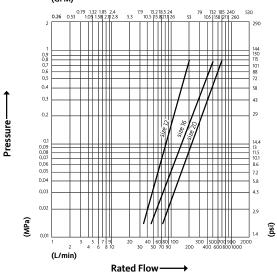
Test performed according to ISO 18869
