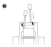
Carefully clean and lubricate the groove. Insert the seal.
