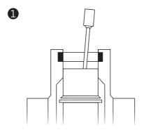
Block the plate in a vice and pull back the valve with a non sharp tool. Keep back the valve.
