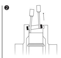
Remove the damaged seal with the help of an hook and pick tool.
