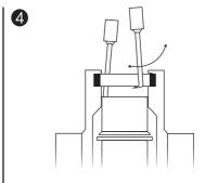
Ensure that the seal is well arranged in its groove and release the valve.
