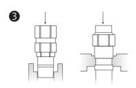
Remove the male coupling from the plate.
