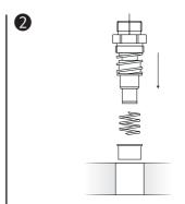
Reassemble the new female coupling.
