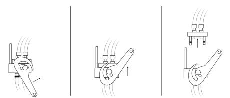
Hold firmly the lever and push the safety button. Lift up the lever till the rolling pins are free from the cams profiles. Place the mobile part on the suitable support. Close the dust protection on the fixed part.
