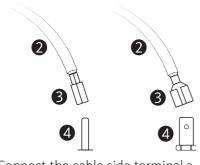
Connect the cable side terminal 3 to the connector side terminal 4.
