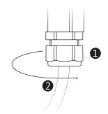
Block the cables 2 with the pressing cable 1.
